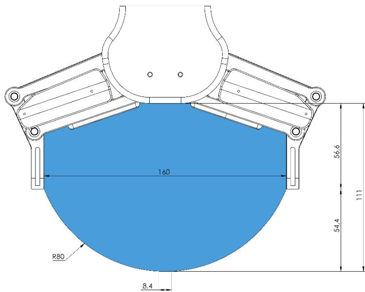
Gripping on long objects can unintentionally activate the Safety switches. The maximum workpiece height (calculated from the end of the fingertips) is dependent on the gripping width (w). For various width values the height (h) limit is given below:
