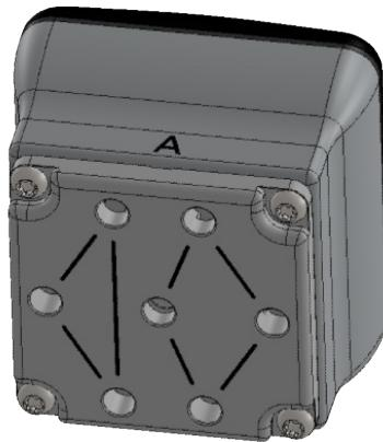
To mount the Adaptor Plate simply remove the 4 fittings or blinding screws from the gripper, place the Adaptor Plate by choosing the right angle according to the desired configuration, and tighten the 4 screws with 4 Nm tighten torque.
