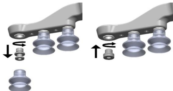
The thread size is the commonly used G1/8"; allowing for standard fittings, blinders and extenders to be fitted directly to the VG grippers.
