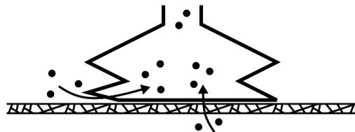
Leaking workpieces can be even harder to identify. Things that look completely tight might not be tight at all. A typical example is coarse cardboard boxes. The thin outer layer is often requiring a lot of air flow to create a pressure difference over it (see figure below).
